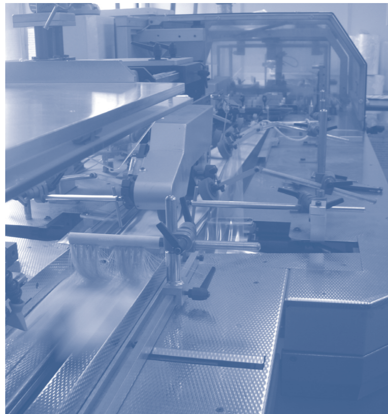
Sitma polywrap workstation with a capacity of 12,000 units per hour
